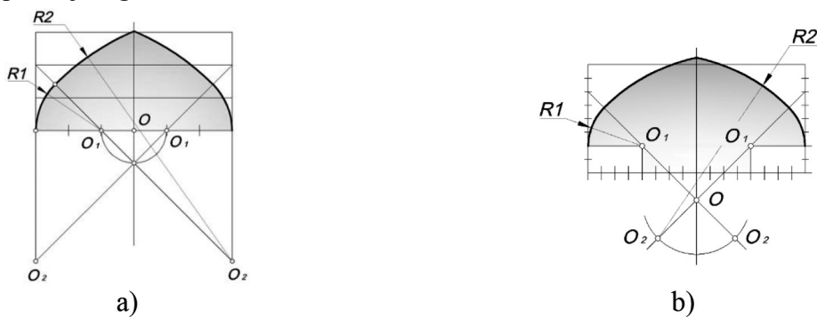
2-rasm. To‘rt markazli arkalarning geometrik yasalishi.
